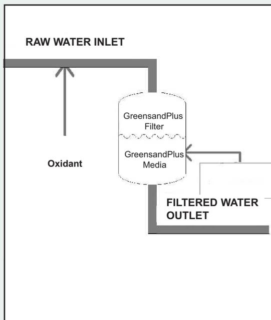
Catalytic Oxidation (CO) operation is recommended in applications where iron removal is the main objective in well waters with or without the presence of manganese. This method involves the feeding of a predetermined amount of chlorine ( $\text{Cl}_2$ ) or other strong oxidant directly to the raw water before the GreensandPlus Filter.
